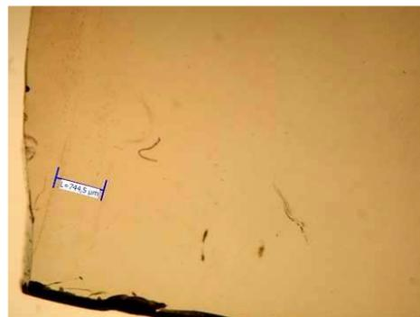
Fig. 2: Induced striation in  $\text{PbCl}_2$  single crystal doped with  $\text{AgCl}$ . Due to insufficient contrast, striations were stressed.
